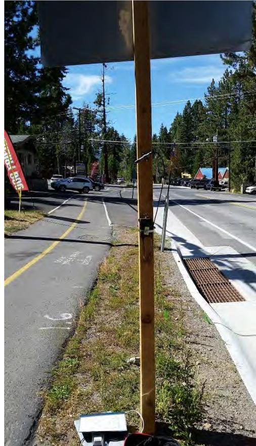
*Left: Passive Infrared Automatic Counter prior to installation. Right: Passive Infrared Automatic Counter installed in the field at the West Shore Bike Path location.*
