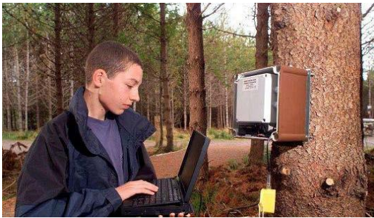
Radio wave detection box and data download Photo Source: Trail Counters
