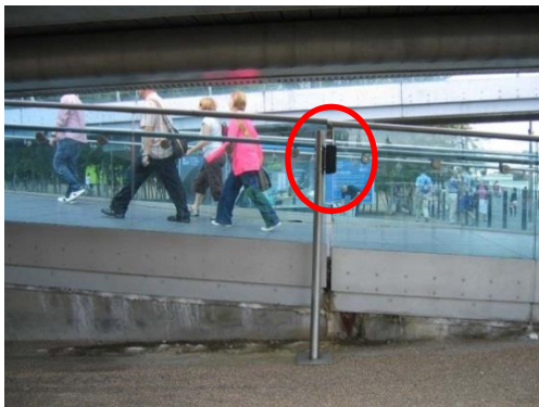
Installed passive infrared sensor Photo Source: Ecocounter
