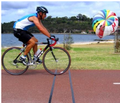
Piezoelectric strips on bike path Photo Source: Metrocount
