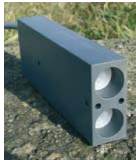
Bi-directional passive infrared sensor Photo Source: Ecocounter
