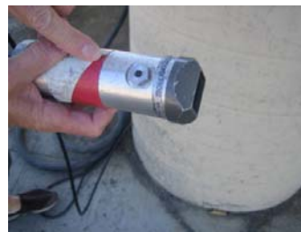
Figure 4: The probe extracts fare and passenger information collected by the GFI system on the vehicle.
