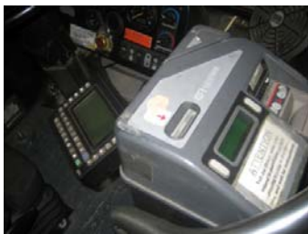
Figure 2: Drivers record the passengers by type on the keypad. The system records the passengers and revenues.
